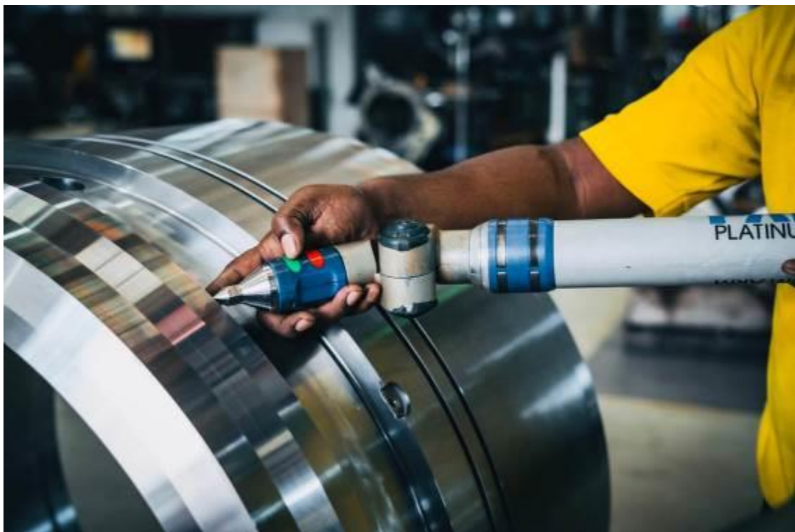
A technician uses a Faro arm to inspect manufactured parts to ensure they meet the specified tolerances. This process demonstrates Fong Lee's dedication to precision and quality.
