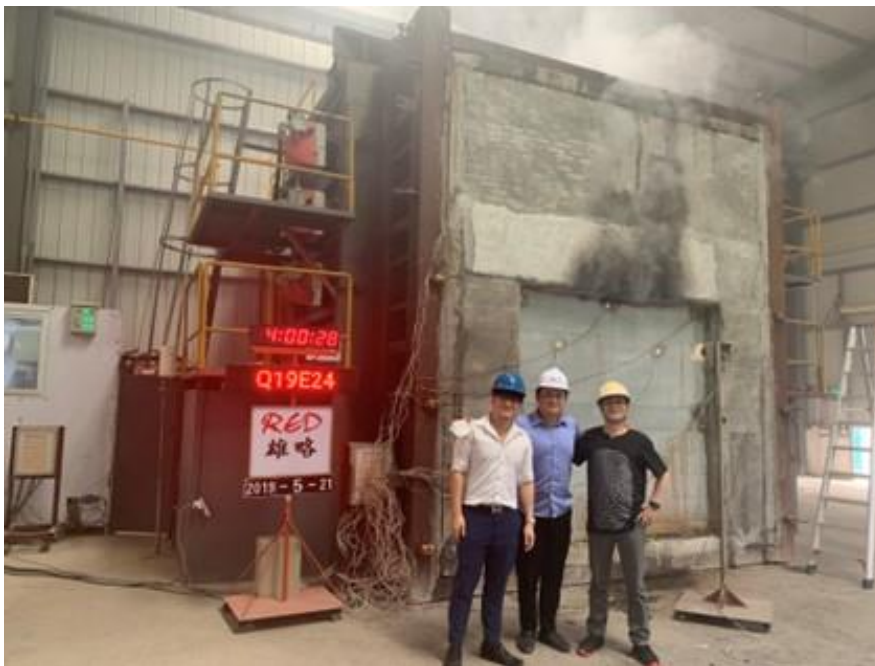
Chua Yong Hin (centre), with his brother, Chua Aik Hin, and their colleague, Xu Shao Hua, attending a European Standard (EN BS 1634) fire certification laboratory test for Delta Technology Pte Ltd's insulated fire shutter, which the company developed in-house in Singapore
